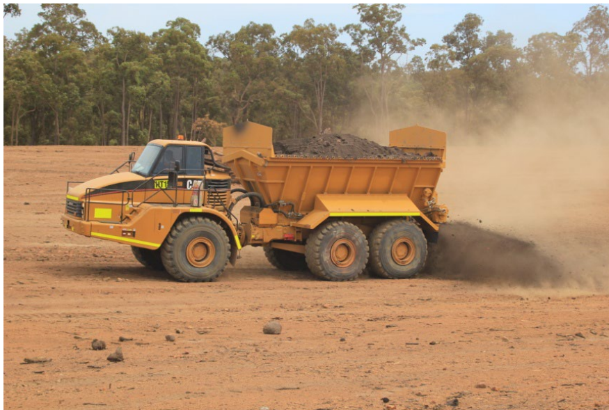
Figure 60. Fresh Topsoil Spreading at Alcoa
