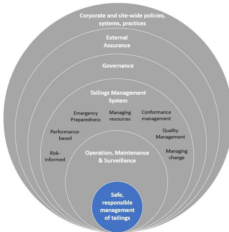
Figure 59. Layers of a Tailings Management System
